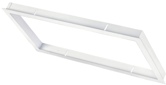
PLASTER RECESS FRAME* (CODE: PRF312) DIMENSIONS: 330MM x 1230MM x 40MM CUT OUT DETAILS: 310MM x 1210MM
