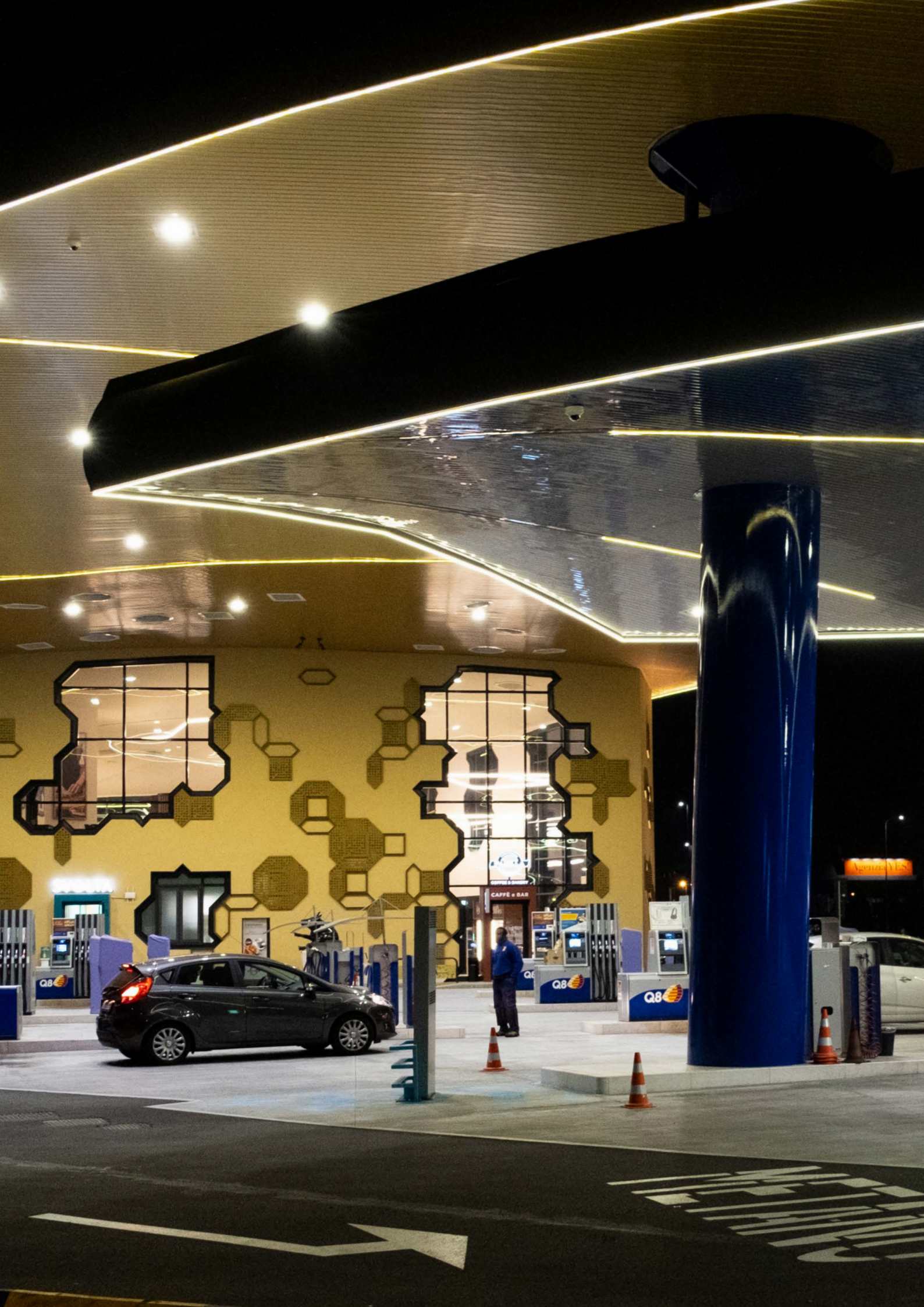
Dot.fuel | Ottica PS | 200lux at 1.65W/m 2
